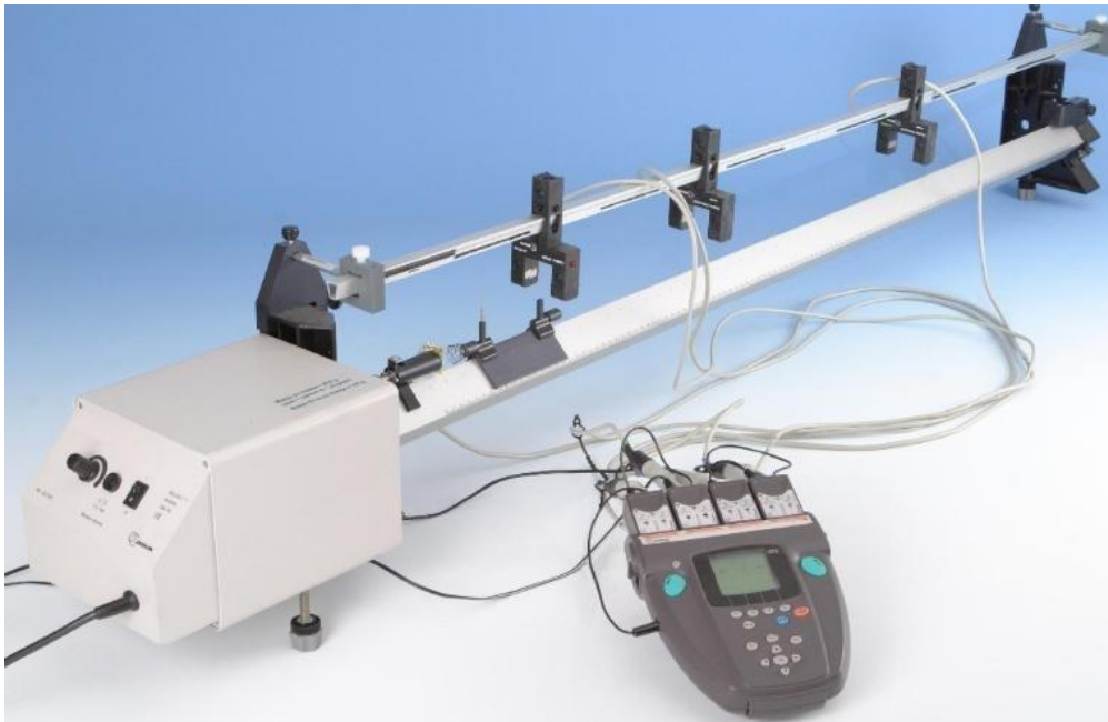
Figure 2. Experimental circuit of Newton's second law in the case of an inclined plane
